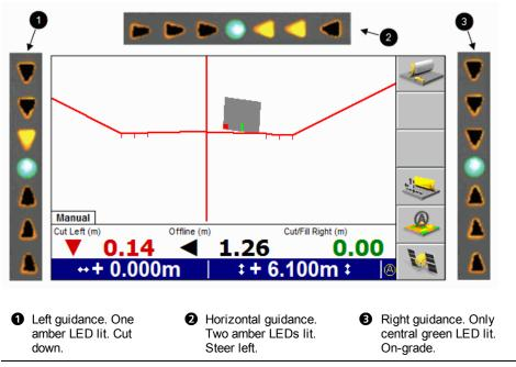
Figure 2.4 Using the 3D lightbars
