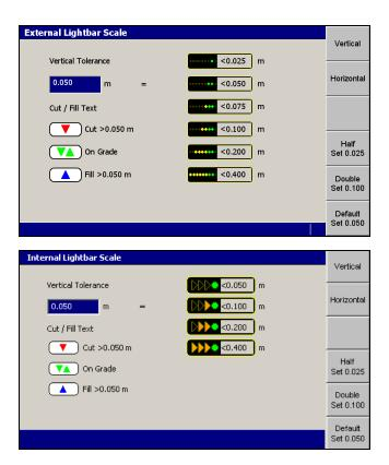
3. Press either **Vertical** or **Horizontal** to view the current vertical or horizontal tolerance settings respectively.
