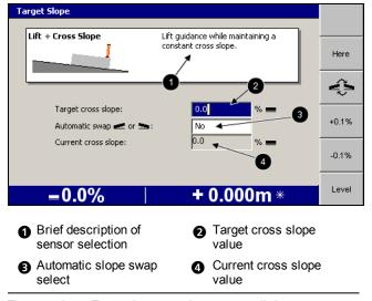
Figure 4.6 Example cross slope setup dialog
