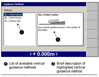
Figure 3.1 Example of a 3D *Guidance Method* dialog
