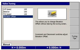
To ensure you keep the blade load constant during tuning, you can change the elevation offset without leaving the tuning screen.
