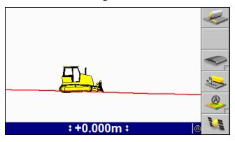
*Note* – The system can be configured for either Split View or for Profile View and Cross-section View. Split View is not available when the system is set for Profile View.
