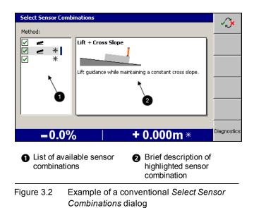
3. Highlight your preferred sets of sensor combinations and press it to enable or disable each selection. This forms a favorites list that can be selected from the guidance screen by pressing the **Sensors** softkey. To open the sensor selection list from the guidance screen, press and hold the **Sensors** softkey.
