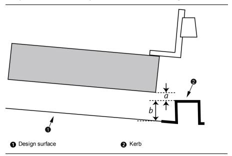
stringline or kerb to the design elevation under the blade tip.
