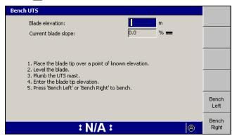
4. Enter the elevation of the benchmark into the Blade elevation field.
