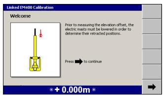
2. Press . The masts are driven to the bottom of their travel range. Once calibration has finished, the *Elevation* screen of the *Linked EM400 Calibration* wizard appears:
