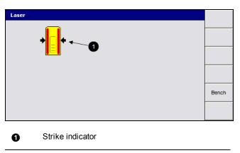
Figure 4.3 Laser strike indication in the *Laser* dialog for a manual mast
