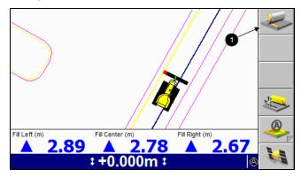
Some softkey labels appear in more than one screen, in which case the function of the softkey they identify is always the same.
