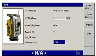
2. Press **Raise Mast(s)** and/or **Lower Mast(s)** to position the mast so that line of sight with the UTS target is maintained, while at the same time keeping the
