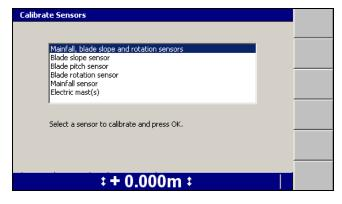
The *Calibrate Sensors* dialog lists the calibration options that are available. The contents of the list depend on the sensors configured for your machine.
