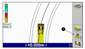
There is difference between **Mapping: Auto** and **Mapping: On**. If configured as **Mapping: Auto**, the system may have more requirements before it will record data. If the system was configured as **Mapping: On** it will always map.
