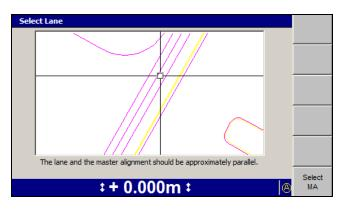
*Note* – *When there is no master alignment in the current design, only the* **Select MA** *softkey is displayed.*
