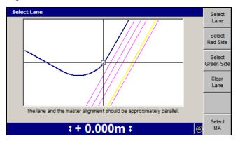
The selected line is shaded double-thick blue and the lane guidance softkeys are displayed.
