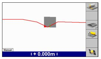
*Note* – *The system can be configured for either Split View or for Profile View and Cross-section View. Split View is not available when the system is set for Cross-section View.*
