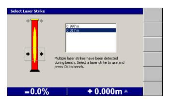
**Note** – By default, laser strikes must be at least 100 mm (4 inches) apart to be distinguished as coming from separate laser transmitters. It may take a few seconds for the system to gather enough data to distinguish between clusters of laser strikes from different transmitters. For this reason, there may be a short delay between pressing the Bench Left or Bench Right softkey, and the appearance of the Select Laser Strike dialog.
