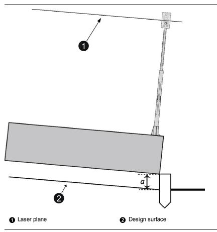
Figure 4.5 Measurements for benching a laser receiver over a benchmark
