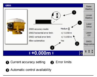
Figure 5.1 GNSS accuracy mode dialog
