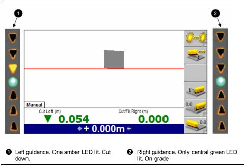
Figure 2.5 Using the 2D conventional lightbars
