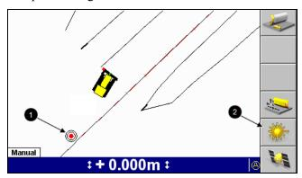
The plan view guidance shows the location of the laser transmitter (**0**):
